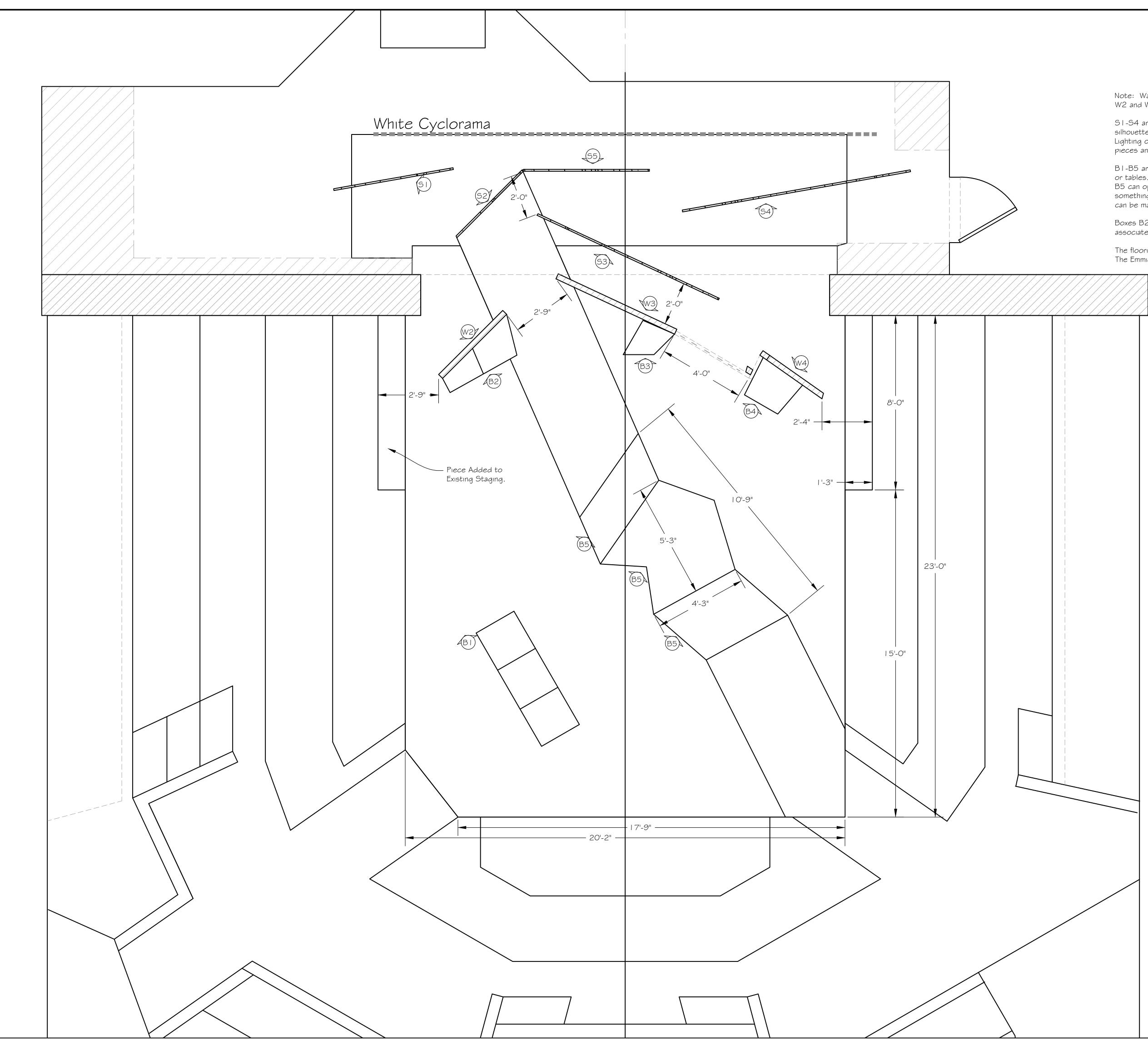
Note: Walls W1-W5 are wood paneled. W2 and W4 Could be movable.
